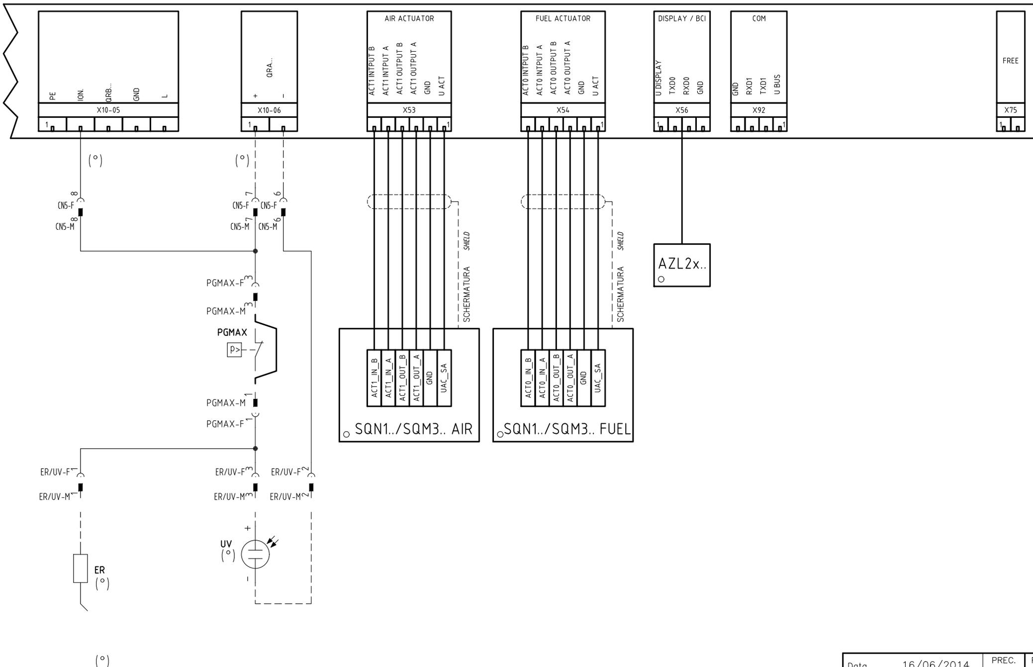
SONDA "UV" IN ALTERNATIVA A ELETTRODO "ER"
