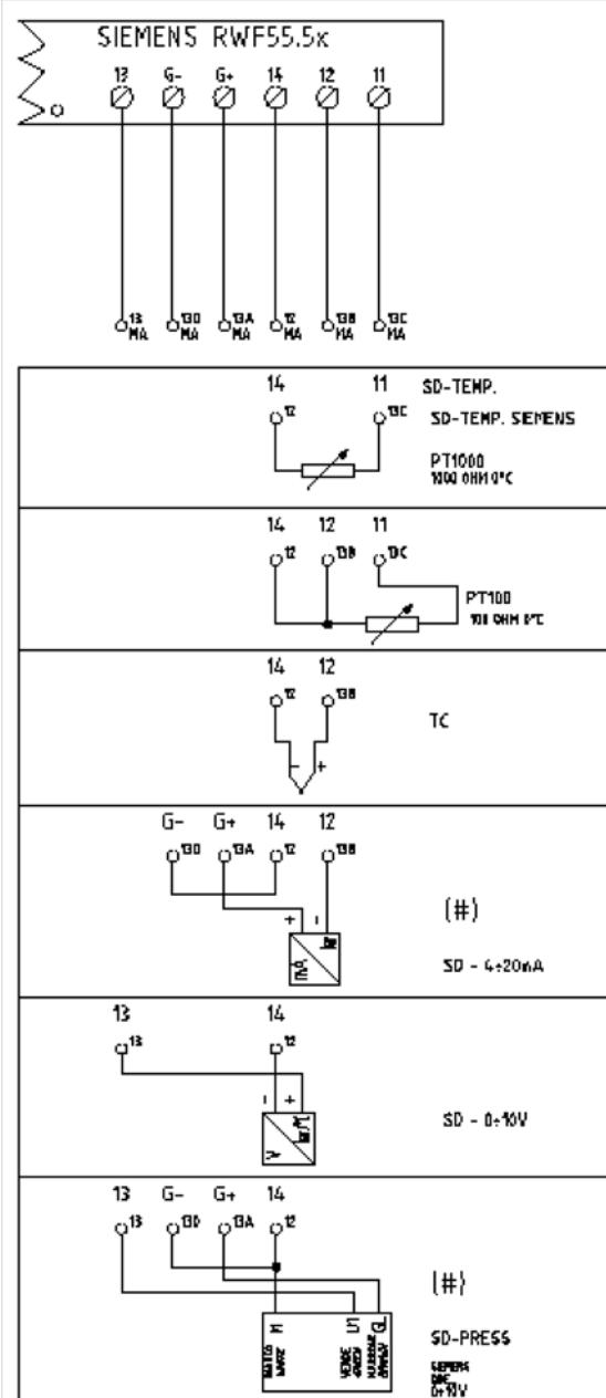
Correspondances bornes entre RWF55.5x y RWF40.0x Correspondence of terminals between RWF55.5x and RWF40.0x
