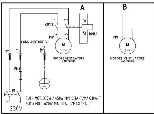
(#) MOTORE VENTIL. VERSIONE [A], FU2 = 6,3A F; MOTORE VENTIL. VERSIONE [B], FU2 = 10A F
