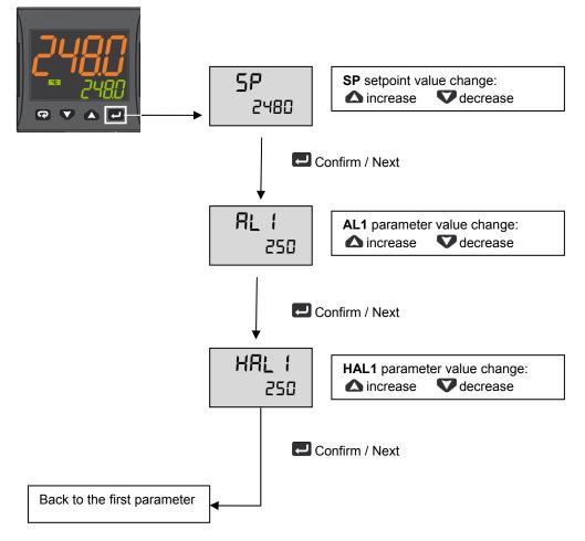
To return to normal mode, press the 😨 key for 3 seconds or wait the 10s timeout
