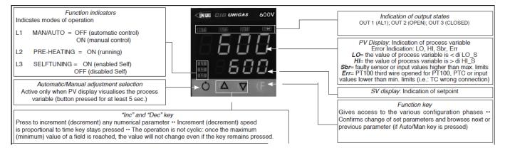
Regulation of the set-point = 80It can be modified by using arrows "up" and "down". By pushing **F** you go to parameters:
