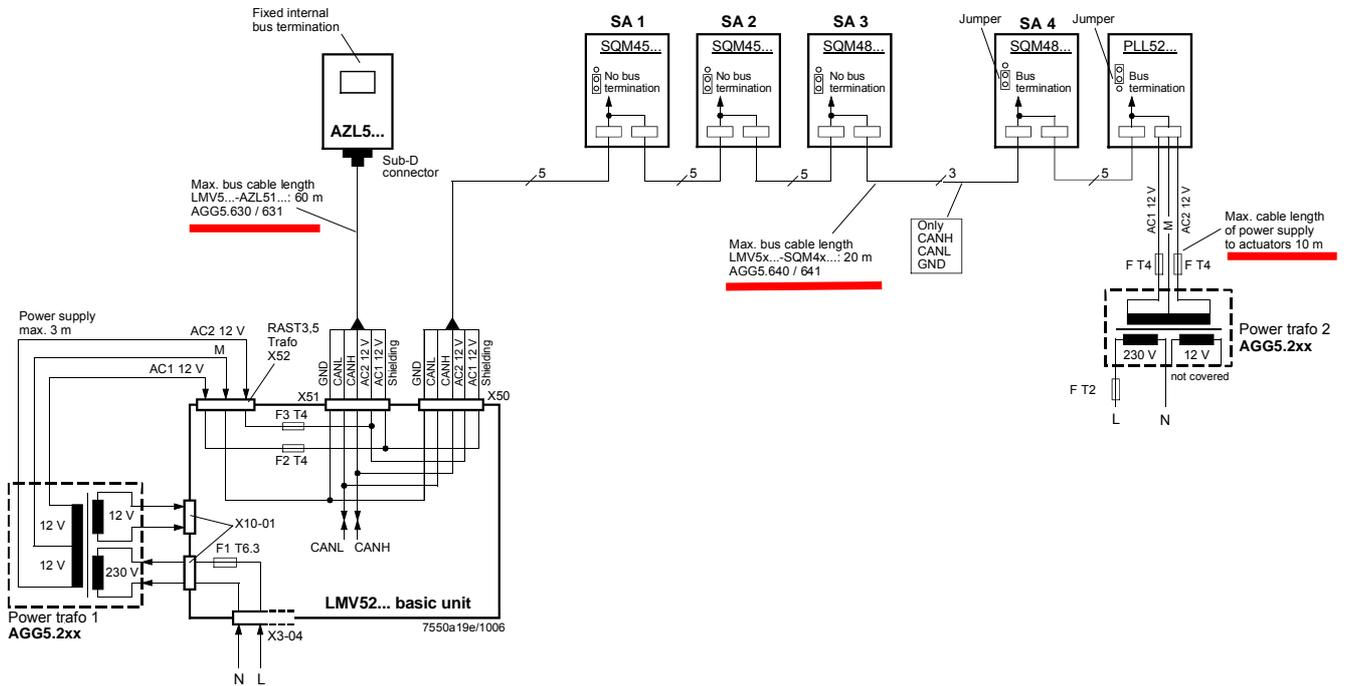
**CAN bus cable with LMV52... and more than 4 actuators and O2 module PLL52...**
