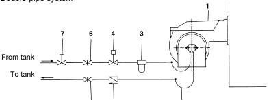
The burner is supplied with filter and flexible hoses, all the parts upstream the filter and downstream the return flexible hose, must be installed by the customer. As far as the hoses connection, see the related paragraph.
