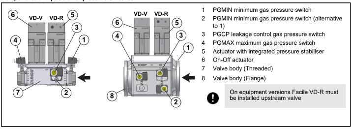
PS pressure sensor connection to VD-R actuator and gas train
