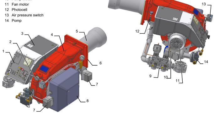
**Gas operation:** the gas coming from the supply line, passes through the valves group provided with filter and governor. This one forces the pressure in the utilisation limits. The actuators move proportionally the air damper and the gas butterfly valve, in order to achieve the optimisation of the gas flue values, as to get an efficient combustion.
