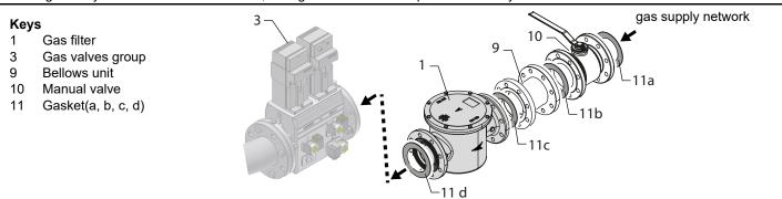
Procedure to install the double gas valve unit: two (2) gas flanges are required; they may be threaded or flanged depending on size
